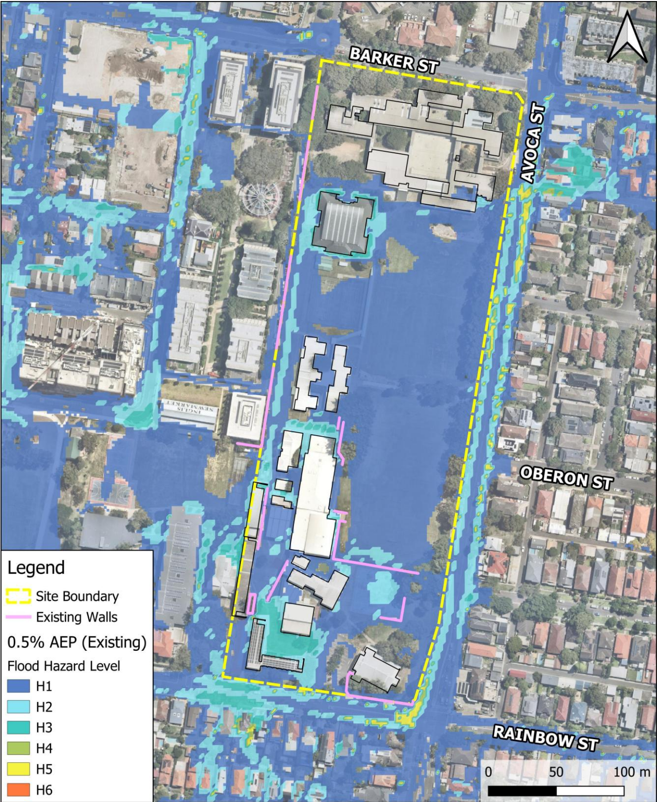
Appendix B 9: 0.5% AEP flood hazard level at Randwick High School under existing conditions
